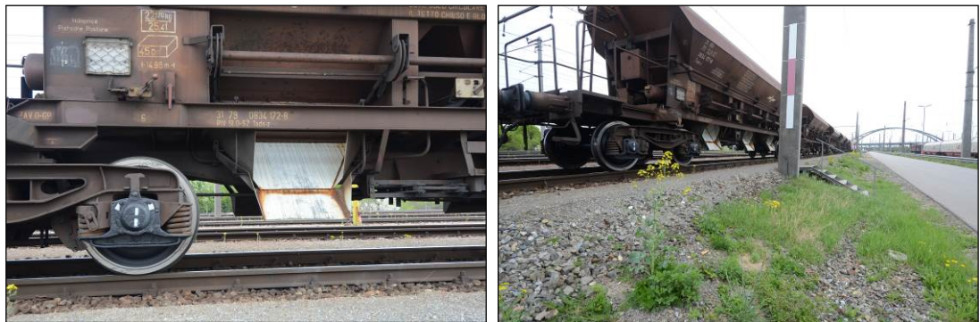
Figure 41: Cleaning area of wagons: a) unloading hatch of wagon; b) feral OSR plant tracing back to seed spillage during cleaning.
